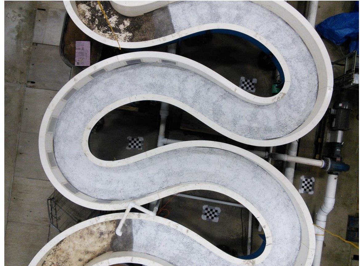
Bedrock bed painted white to increase contrast between bed and alluvium.
