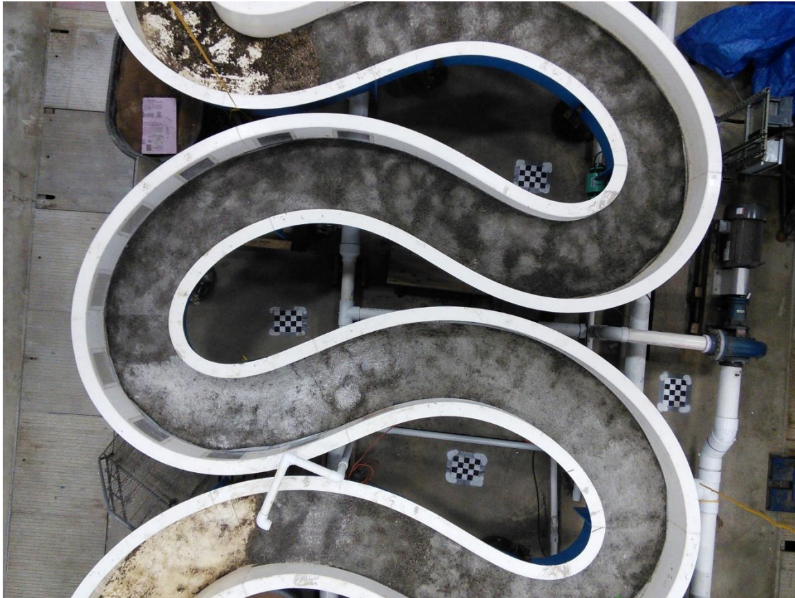
Flume with bedrock bed (all gravel and foam covered with thin layer of concrete).
