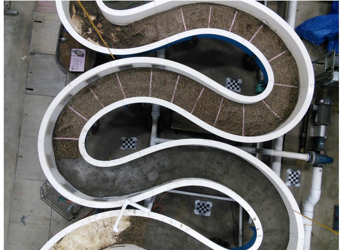
Flume with foam cross sections, gravel and thin layer of concrete between CS7 and CS14
