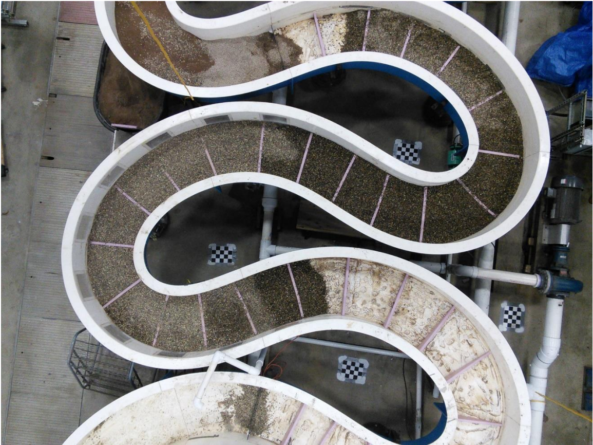
Flume with foam cross sections and gravel filling the pockets between XSs
