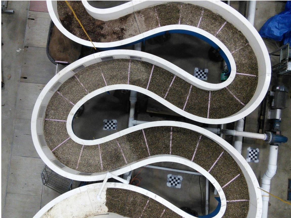
Flume with foam cross sections and pockets fully filled with gravel
